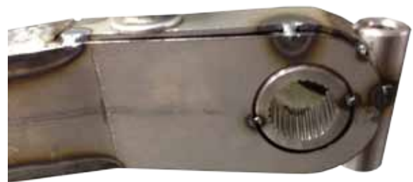
Pro Fabricator Link Arm tacked together
